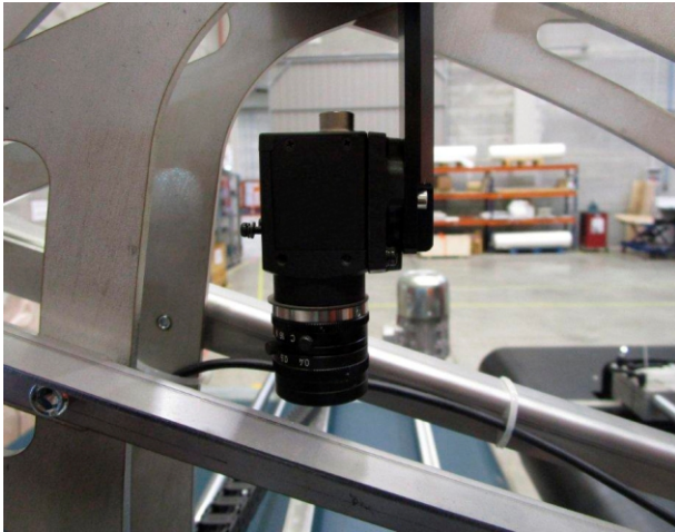
The EFI Cretavision 2.0 compact camera in place
